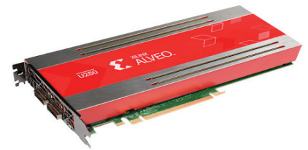
Figure 4: Xilinx Alveo data center FPGA accelerator
