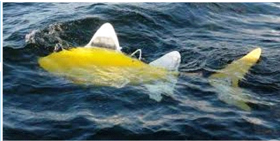
Figure 3: SHOAL robotic fish detects underwater pollution. (Picture Credit: InfoNIAC website)
