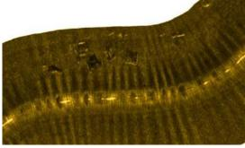
The accident of the MV X-Press Pearl caused a massive threat to the safe operation of the Colombo Port. Due to this incident, many containers and debris might have fallen into the navigation channel and an urgent hydrographic survey was conducted in July 2021 to confirm the clearance for safe navigability. A detailed Side Scan Sonar (SSS) survey was conducted
